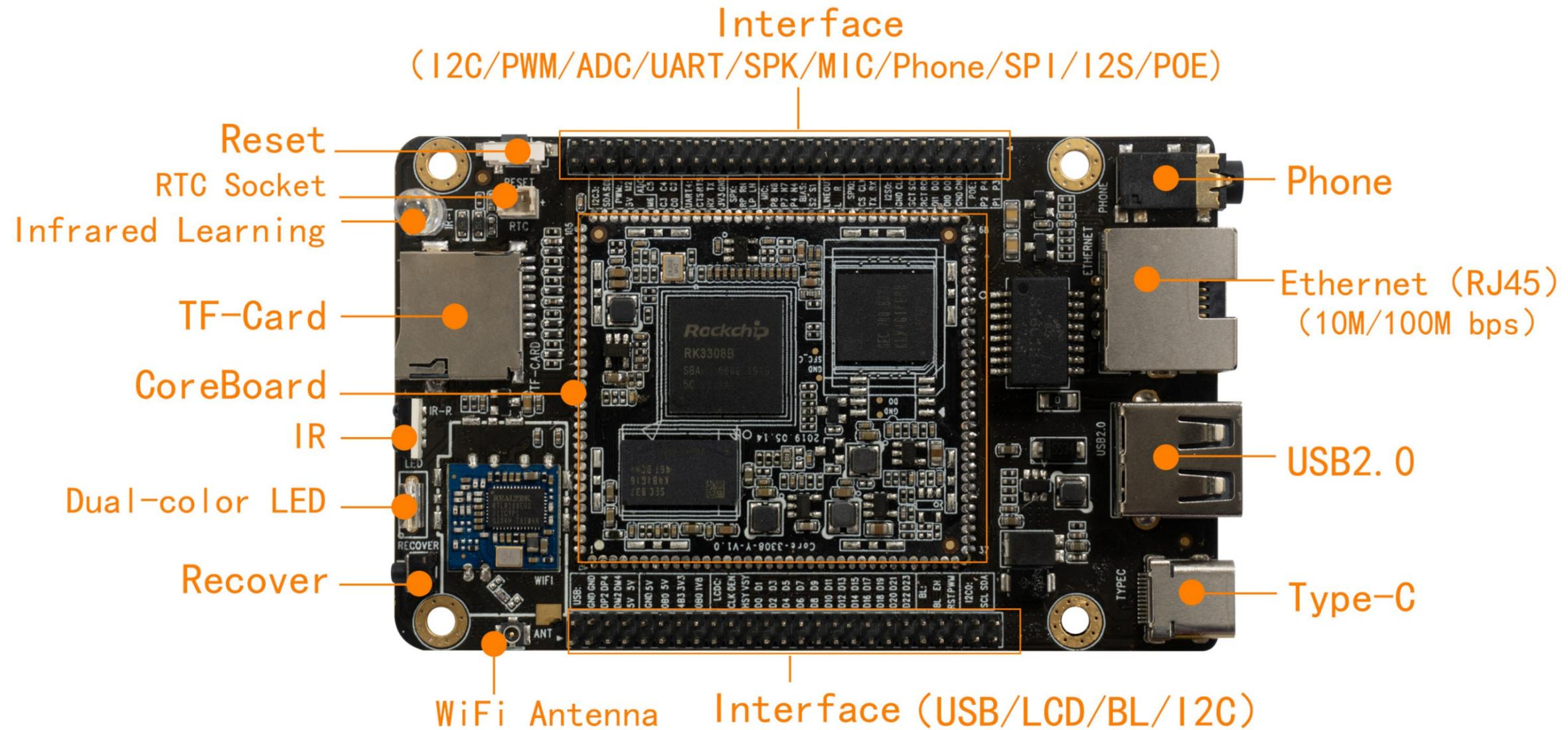
ROC-RK3308B-CC-PLUS (Core Board + Main Board)
