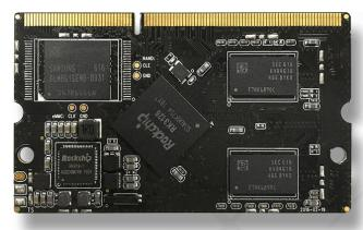
The core board is equipped with immersion gold (IMG) interface which is stable and reliable. The DDR3-204P interface can connect to all the chips, which best guarantees the data transmission and extensibility. The IMG pins are corrosion resistant, solid and reliable as is bolted.
