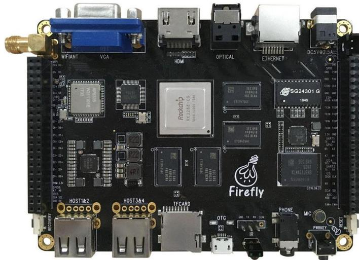
It supports multiple network interfaces: WiFi 2.4GHz/5GHz Dual-Frequency (802.11a/b/g/n/ac protocol), Bluetooth4.1, Gigabit Ethernet, it can be connected to 3G and 4G mobile communication modules through USB interface. Rich extension interfaces: support PWM, PWM, SPI, UART, ADC, I2C, I2S, GPIO.
